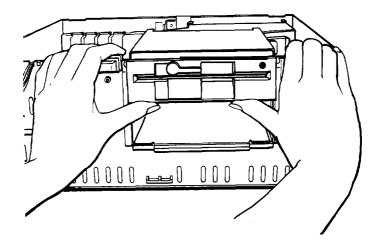
7. Lift up the front of the subassembly with your thumbs. Raise it to a slight angle, as shown below.
